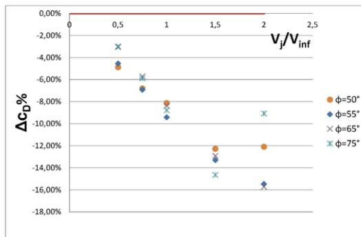
Figure 2: Drag reductions with control of rear part.
