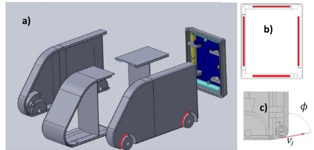
Figure 1: a) Exploded view of modular model for wind tunnel test. b) Jet slots disposition in rear part of the model. c) jet orientation angle.
