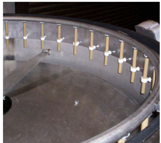
Figure 2: Whirling Arm Rain Erosion Testing at the University of Limerick
