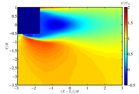
Figure 2: Mean streamwise velocity of the controlled flow.
