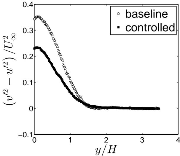
Figure 4: Turbulence anisotropy at  $(X - L_f)/H \approx 1.67$ .
