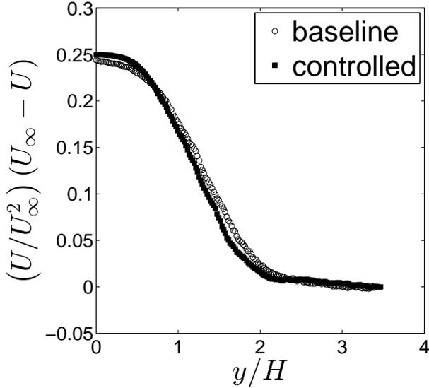
Figure 3: Mean velocity deficit at  $(X - L_f)/H \approx 1.67$ .
