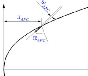
Figure 3 Geometrical optimization parameters of the slit
