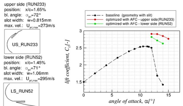
Figure 4: Results of optimized ZNMF for upper and lower side actuations on the DLR-F15LLE airfoil
