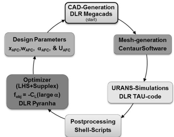
Figure 1: Optimization loop for ZNMf-actuation
