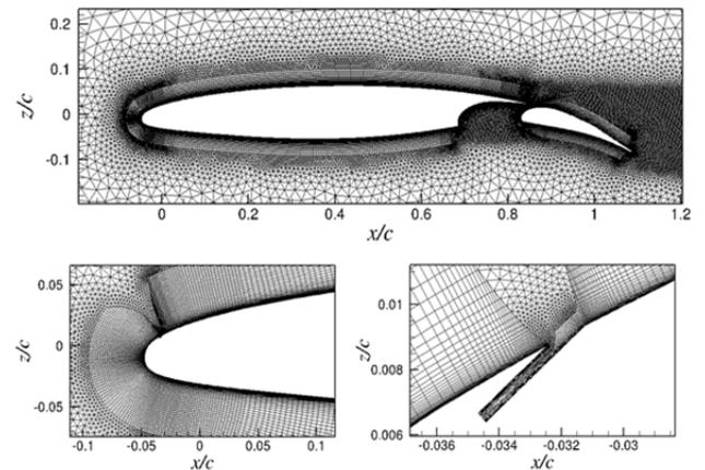
Figure 2: Mesh topology for the 2-elem. DLR-F15LLE including a modeled actuation slit at the leading edge of the laminar airfoil
