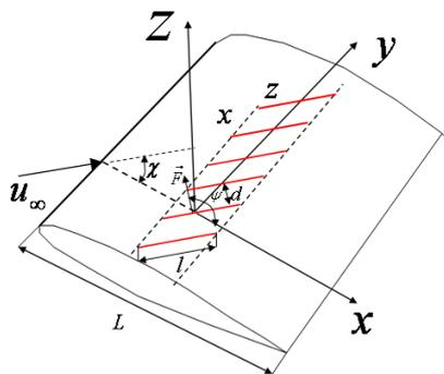
Fig 1. Scheme of multi-electrode DBD actuator
