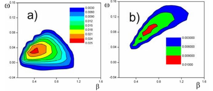
**Fig 3.** Growth rates of unstable disturbances  $\sigma = -\text{Im}(\alpha)$  in oncoming boundary layer (a) and in averaged flow above the actuator with  $\psi=115^\circ$  at  $x=0.6$ m.
