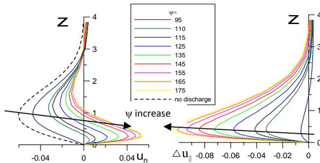
**Fig 2.** Averaged over the span profiles of cross-flow velocity (a) and increment of tangential velocity (b) in the boundary layer at  $x=0.55$ m for different electrode inclination angle  $\psi$
