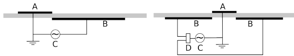
Figure 1: Schematic of the L type (left) and \Pi type (right) plasma actuators. A is the upper electrode; B is the lower electrode; C is the AC power source and D is the phase controller.
