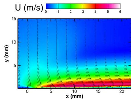
Figure 1: Velocity field produced by a single DBD.
