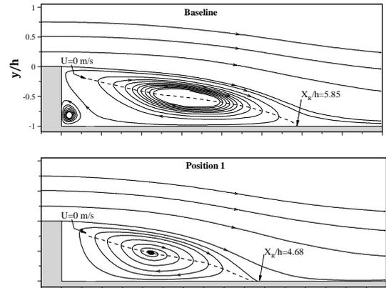
Figure 6: Streamlines of the flow downstream a backward-facing step with and without actuation.
