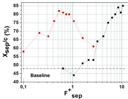
Figure 5: Separation location versus frequency actuation in steady mode (■) and burst mode (●).
