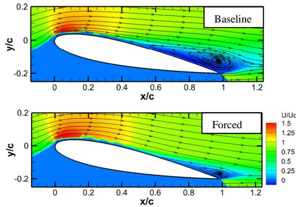
Figure 4: Flow control by DBD ( $Re = 1.33 \times 10^6$ ).
